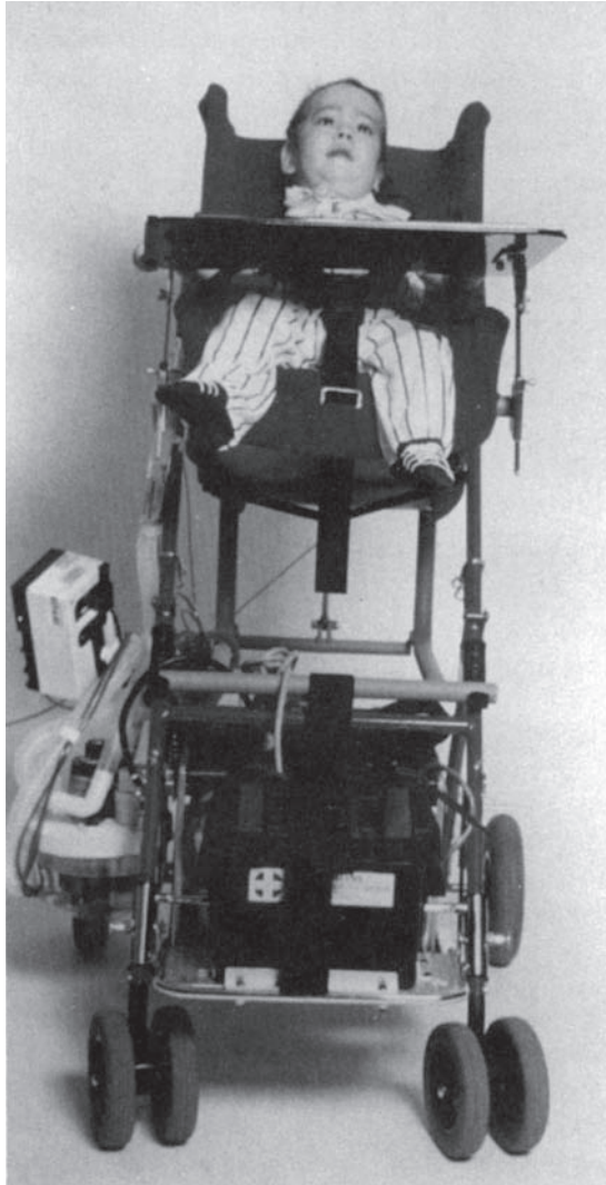
FIGURE 12.16 A Snug Seat adapted for a ventilator.
